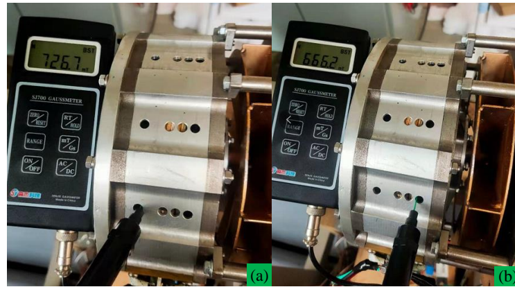
Figure 20. Measurement of flux density of air gap, (a) drive end side, (b) non-drive end side.
