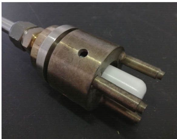
Figure 27. Testing of Pt-air sensors 1100 mm long in oxygen-saturated Pb in the range 350–480 °C.
