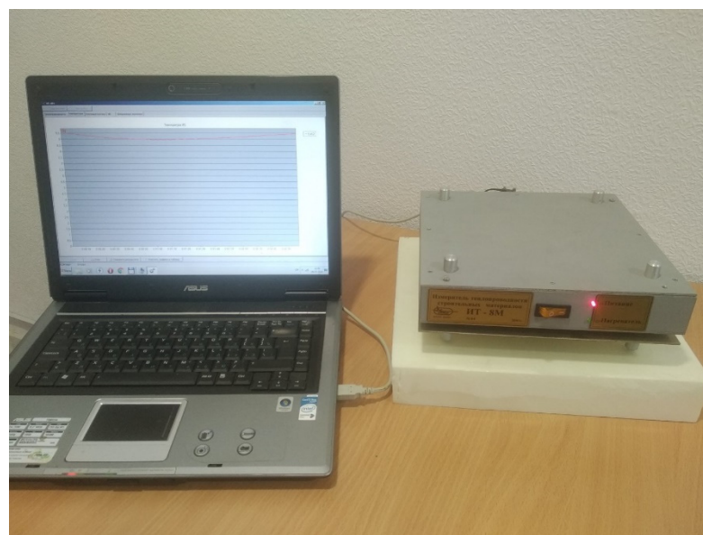
Figure 1. Portable device for the express control of thermal conductivity.
