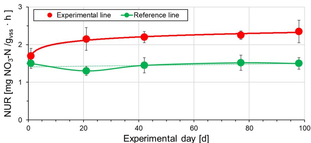
**Figure 2.** Denitrification rates measured in laboratory conditions for biomass from the experimental line (with fusel oil dosing) and reference line (without dosing of fusel oil) at Poznan WWTP.
