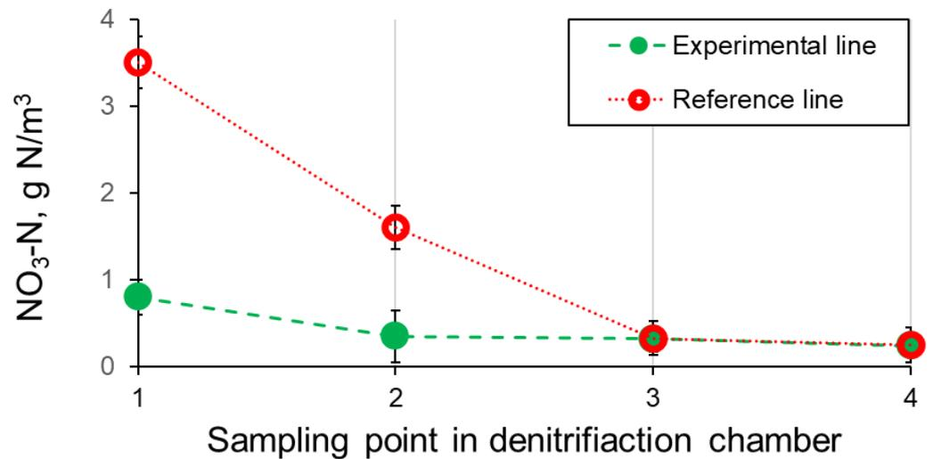
**Figure 3.** Variability of NO<sub>3</sub>-N concentrations in the anoxic chamber in experimental and reference line at Poznan WWTP (average values from the entire research period).
