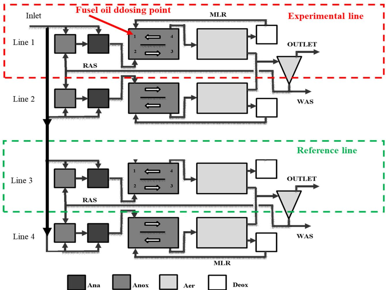
**Figure 1.** Layout of the full-scale JHB systems for investigating the acclimation of biomass to fusel oil at Poznan WWTP. Abbreviations: RAS—recirculated activated sludge, MLR—mixed liquor recirculation, WAS—waste activated sludge. Reactors: Ana—anaerobic, Anox—anoxic, Aer—aerobic, Deox—deoxidation of the MLR.
