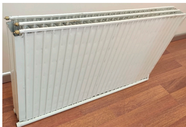
Figure 15. Photo of the Prototype Enover Heat-Pipe Radiator (HPR). This prototype was tested in certified labs.
