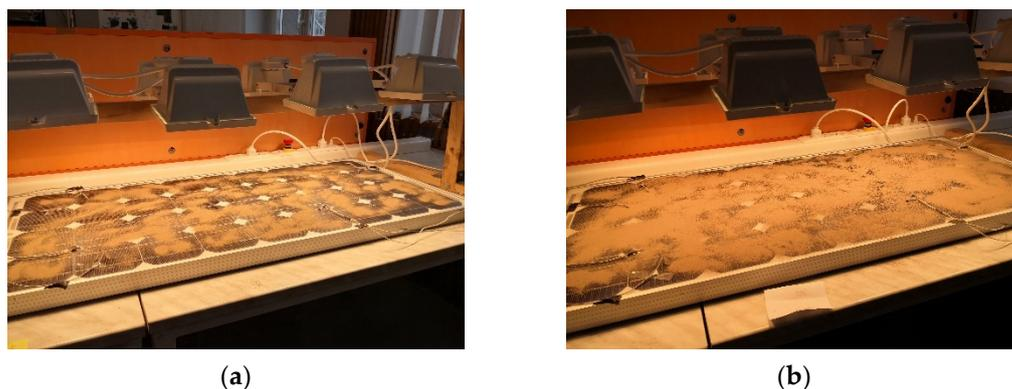
**Figure 3.** Sand-contaminated solar panel (a) and fly ash-contaminated solar panel (b).
