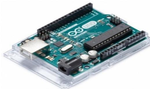
Figure 3. Arduino UNO microcontroller.
