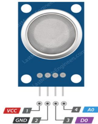
**Figure 7.** Specification and layout of Smoke Sensor.
