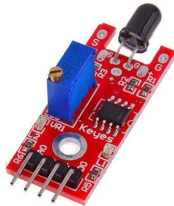
Figure 5. Flame Sensor used in SMDD.
