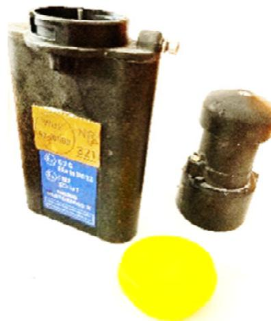
Figure 4. CIP-10R personal dust meter for measuring the PM4 dust respirable fraction of.
