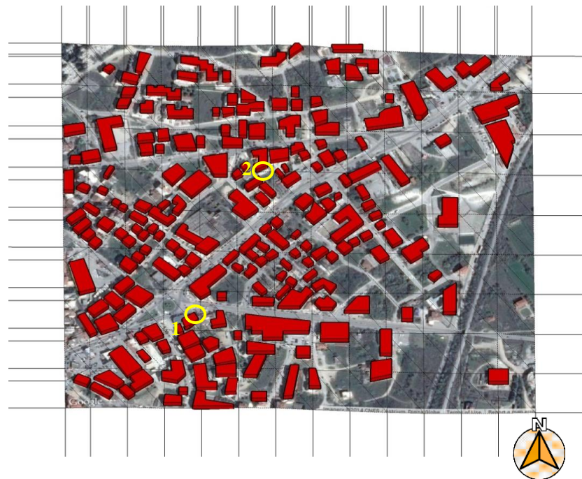
Figure 1. 3D representation of urban area being studied. Measurement positions are also indicated (1) for temperature measurements and (2) for wind measurements. (Satellite view of the city from Google Earth).
