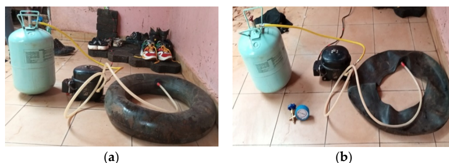
Figure 3. Compression of biomethane (a) full and (b) empty balloon.
