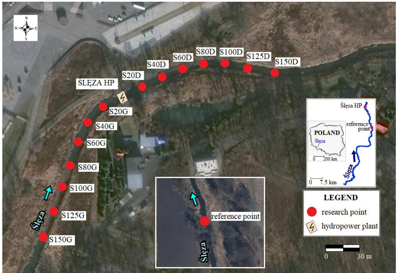
Figure 1. Sediment sampling points of the hydropower plant in Wrocław on the Śleza River.
