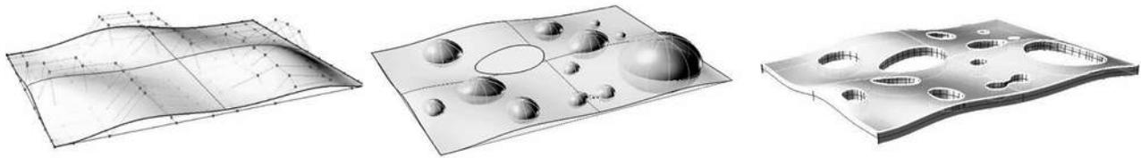
**Figure 6.** Modelling (step by step) the geometry of the free surfaces with Rhinoceros CAD software—initial concept design.
