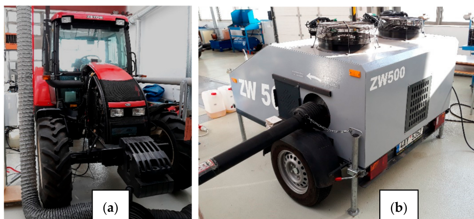
Figure 3. Tractor and the dynamometer used for the measurements: (a) Zetor Forterra 8641, (b) MAHA ZW500.
