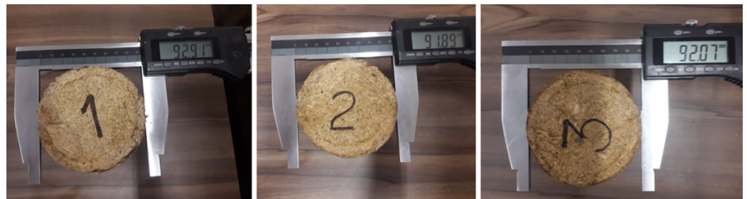
Figure 7. Produced briquettes have a variation in diameter, although perfectly normal.
