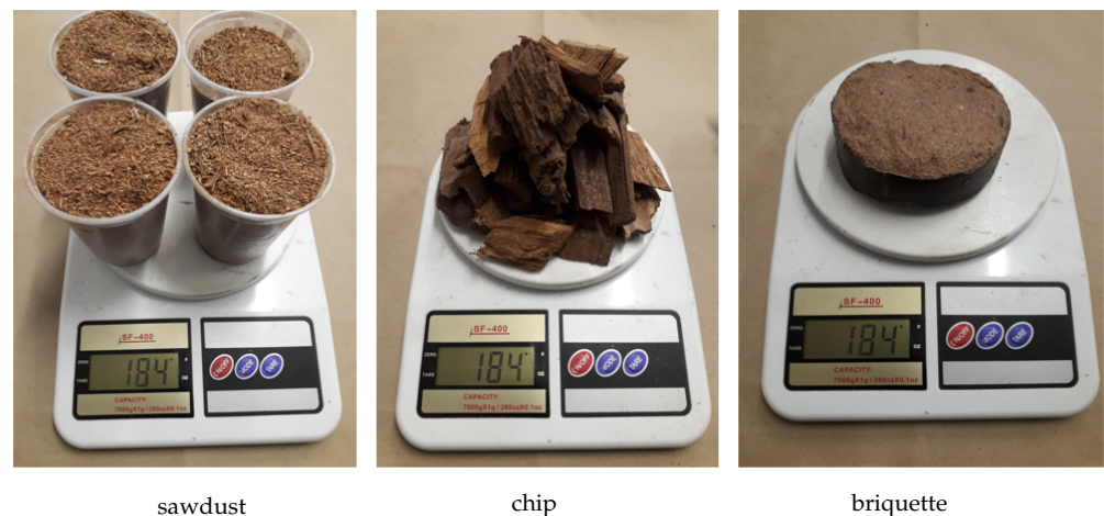
Figure 3. The same amount of biomass in bulk format and in its compacted form.
