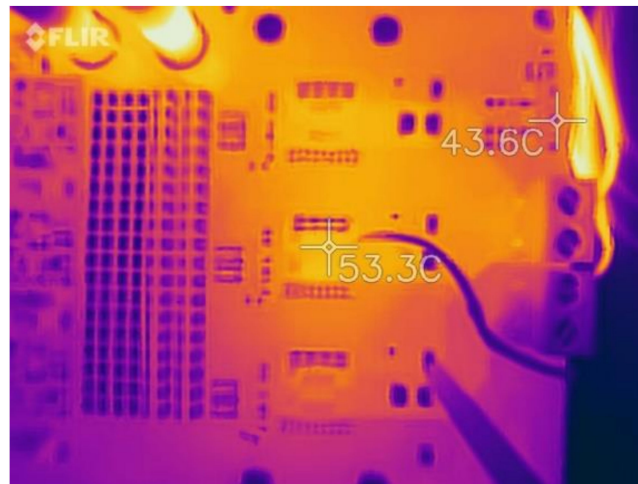
Figure 29. Infrared picture of experimental board without heat sink at V_{dc} = 48\text{ V} , I_{a,b,c,rms} = 10\text{ A} , f_{sw} = 50\text{ kHz} .
