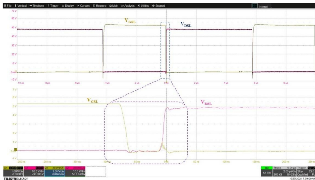
Figure 25. Experimental waveforms of the gate-source voltage of the lower device of inverter leg (phase a) under the rise of the inverter leg node voltage (lower device-drain-source voltage). The dv/dt effect acts a gate voltage spike under the GaN threshold voltage ( V_{GSTH} ) V_{DSL} = 10 V/div, V_{GSL} = 1 V/div, t_{main} = 2 \mu s, t_{zoom} = 50 ns/div.
