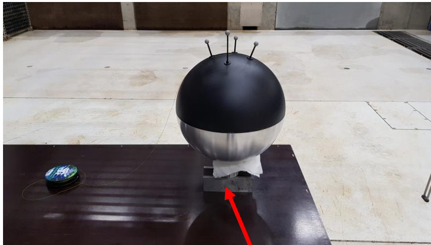
Placing the sphere on blocks exactly 50.00 mm high
