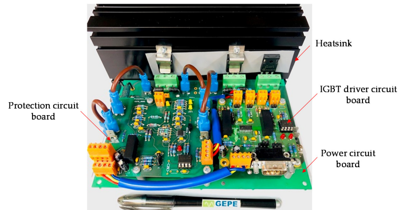
Figure 11. Final submodule (SM) structure.
