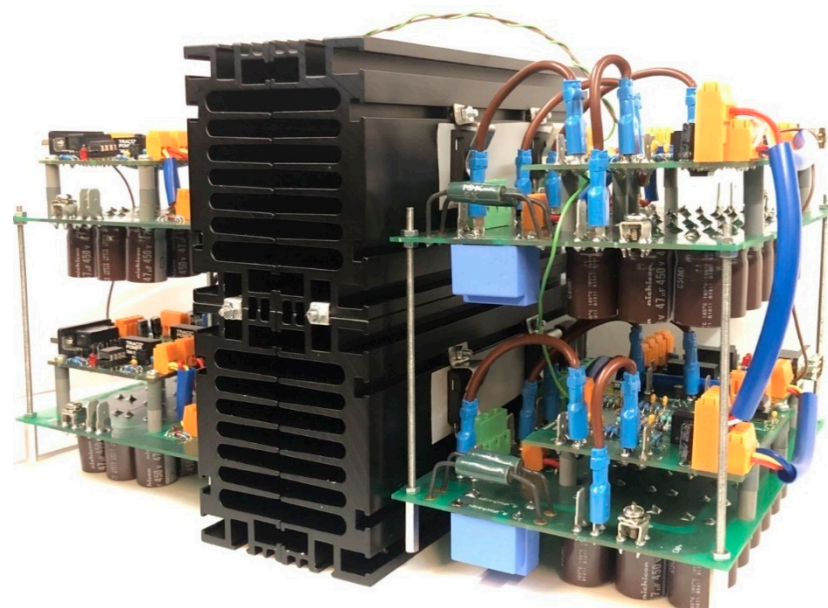
Figure 12. Single MMC leg/phase (four submodules).
