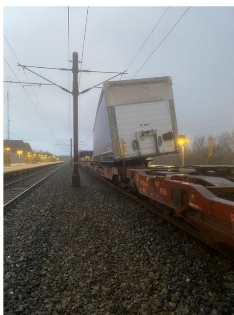
Figure 1. In 2021 during the passage of a freight train over the bridge, the semi-trailer was forced out of its attachment (strong wind and empty trailer), source: utk.gov.pl (accessed on 11 October 2021) [8].
