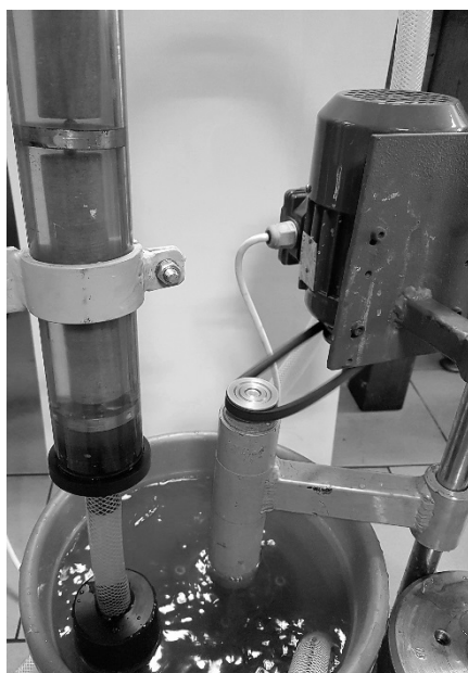
Figure 1. A photo of the drilling fluid flow simulator [27].
