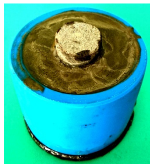
Figure 4. Sandstone core with cement slurry prepared for adhesion tests on the contact surface between the core and cement.
