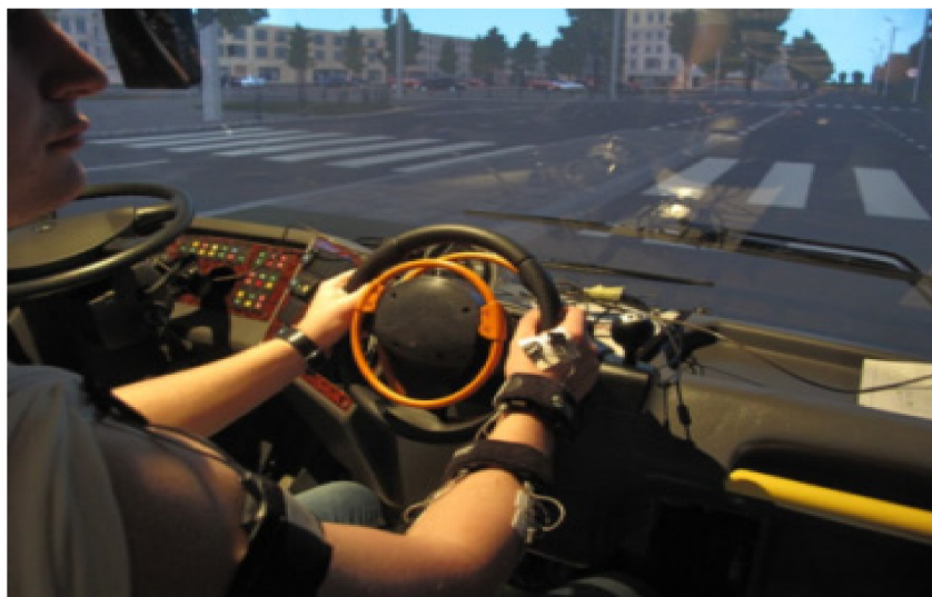
Figure 6. Location of electrodes for surface EMG measurement used in the experiment.
