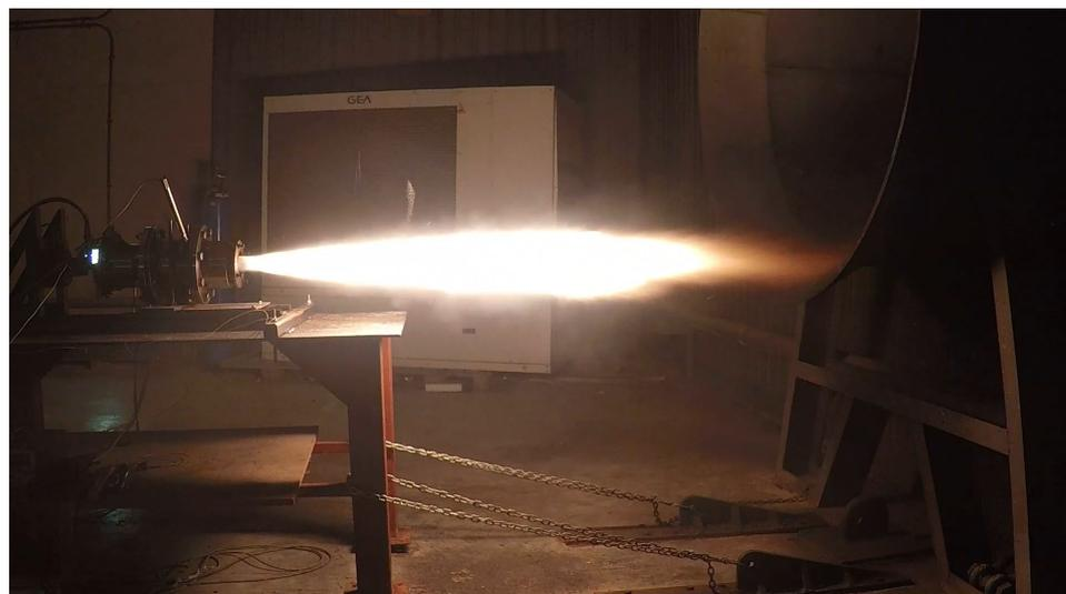
**Figure 4.** The ULB-HRM during operation [7].
