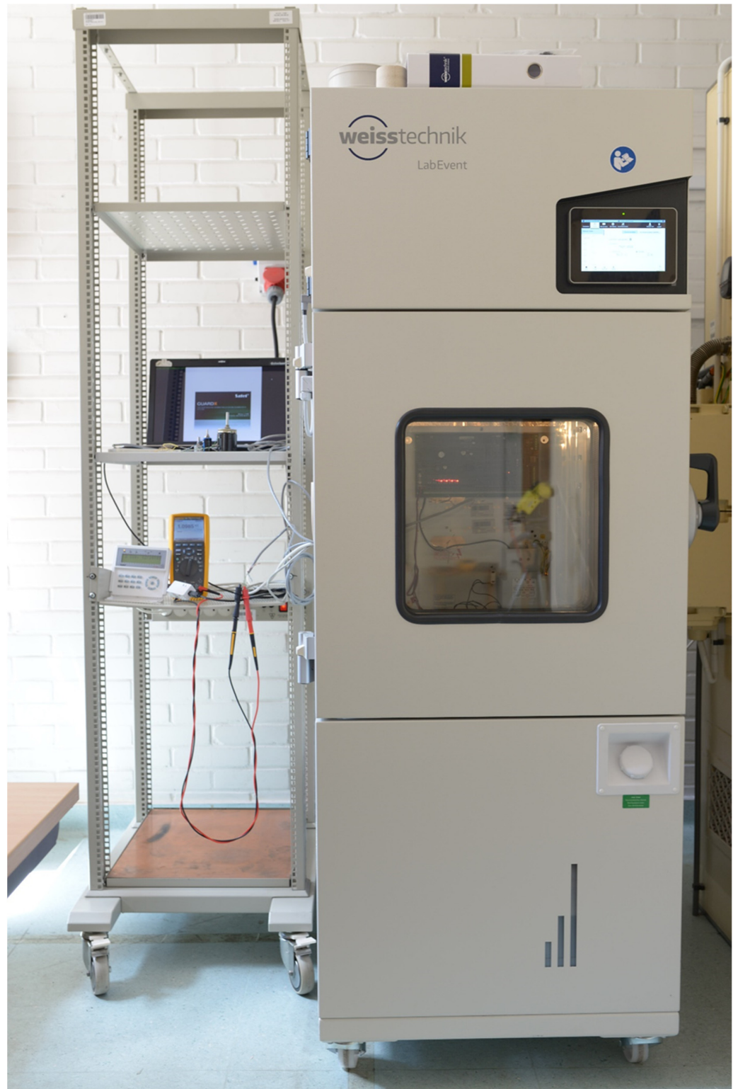
Figure 3. Test bench for studying the impact of temperature on the tripping thresholds of intrusion detection system detection circuits.
