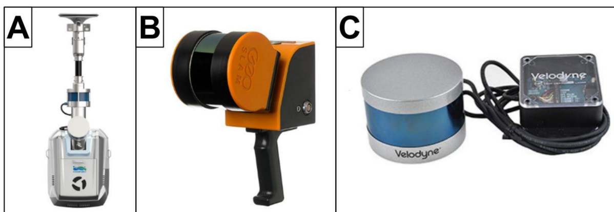
Figure 6. Examples of LiDAR-based scanning systems: (A) GreenValley International LiBackpack DGC50, (B) GeoSLAM ZEB Horizon, (C) Velodyne VLP-16 with an interface box.
