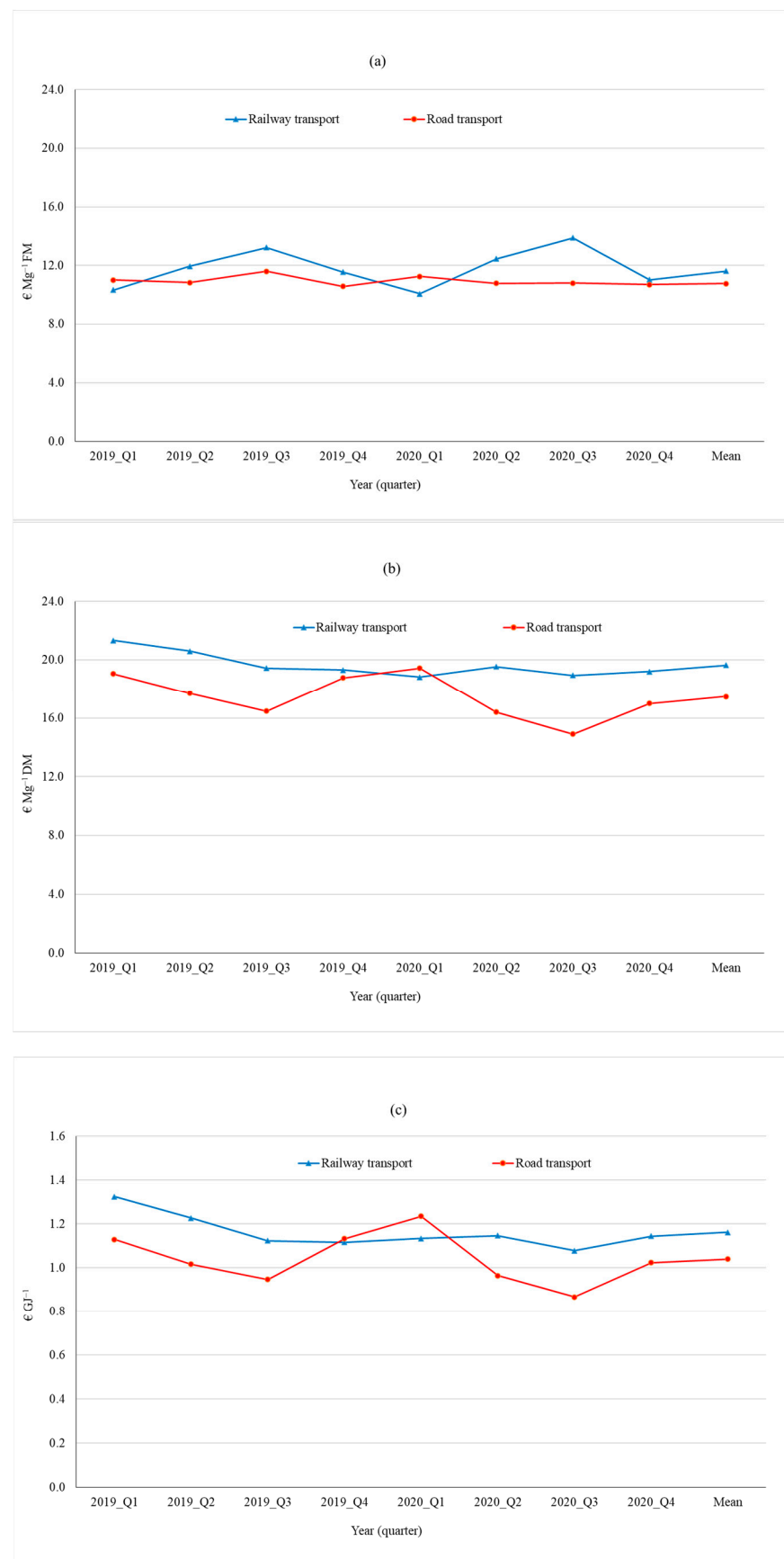
Figure 3. Cost of wood chip transport depending on the year, quarter and transport type concerning (a) 1 Mg FM (fresh biomass), (b) 1 Mg DM (dry biomass), (c) 1 GJ of energy in this solid biofuel.
