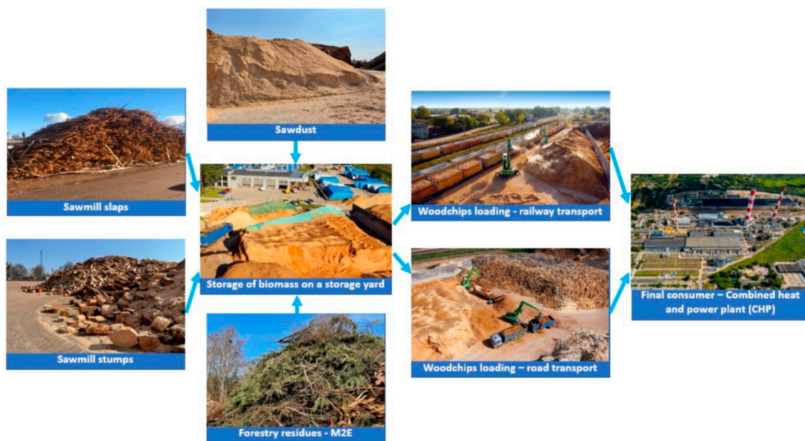
Figure 1. Diagram of wood chip preparation from various types of wood biomass stored at the Quercus site and the logistics of wood chip transport to the end consumer.
