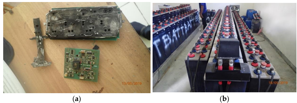
Figure 12. (a) IGBT failure in PV site 2 (b) Battery failure in PV site 3.
