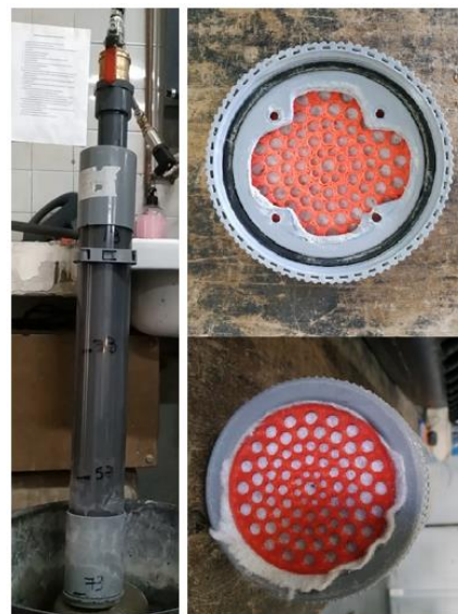
Figure 5. Left, PVC glass tube. Right, perforated and printed pieces.
