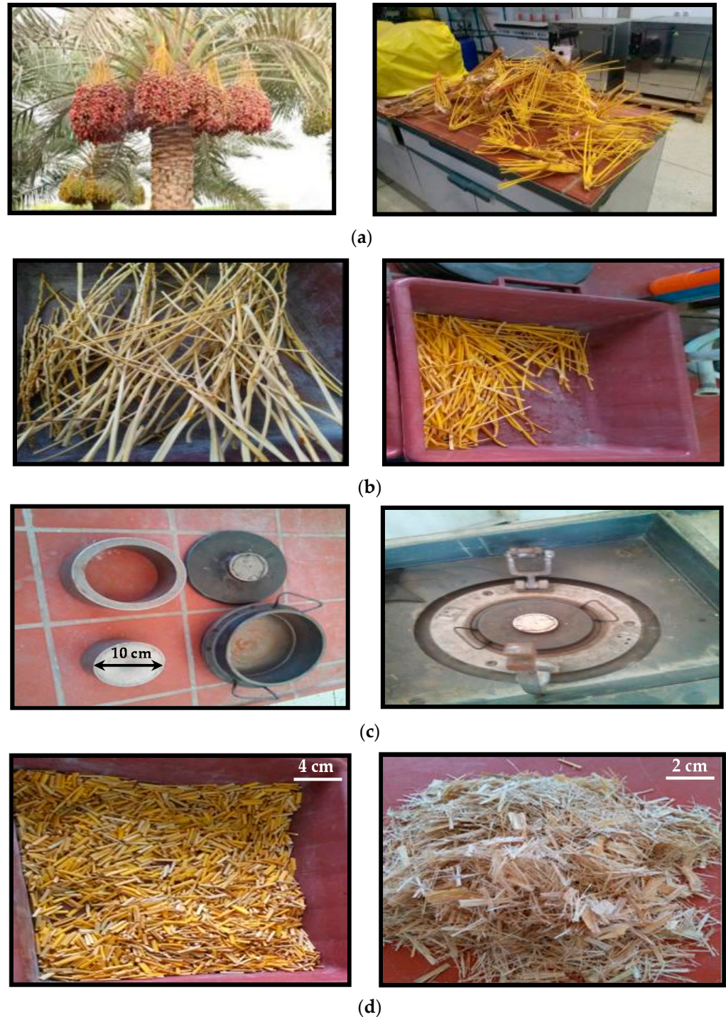
Figure 2. Different extraction steps of palm fibers. (a) Salvaged date stems; (b) cut palm stalk; (c) mill components; (d) palm stem fibers.
