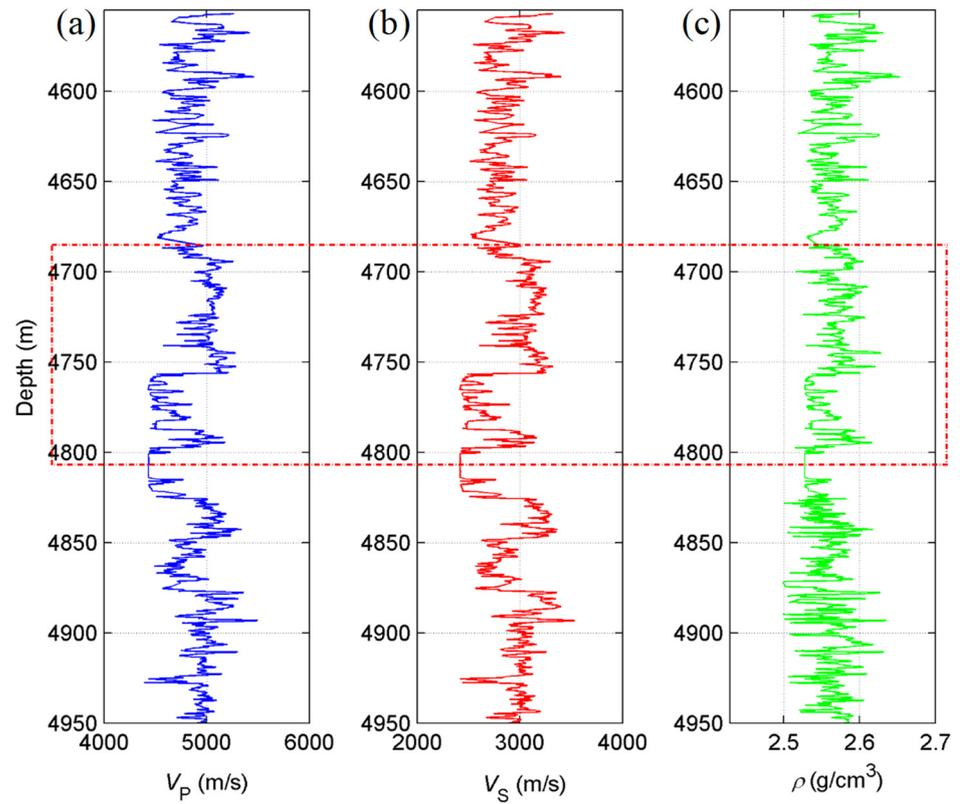
Figure 2. Log profiles of Well P. (a) P-wave velocity, (b) S-wave velocity, and (c) density.
