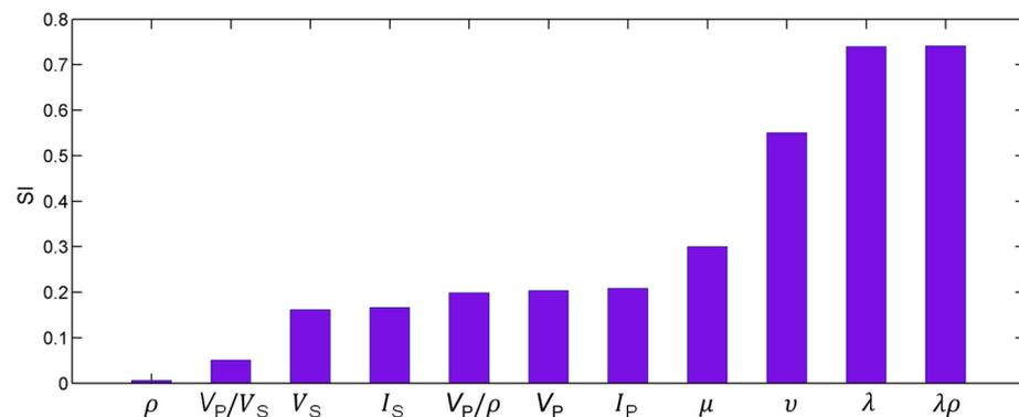
Figure 10. Sensitivity indices varying with the microcrack porosity.
