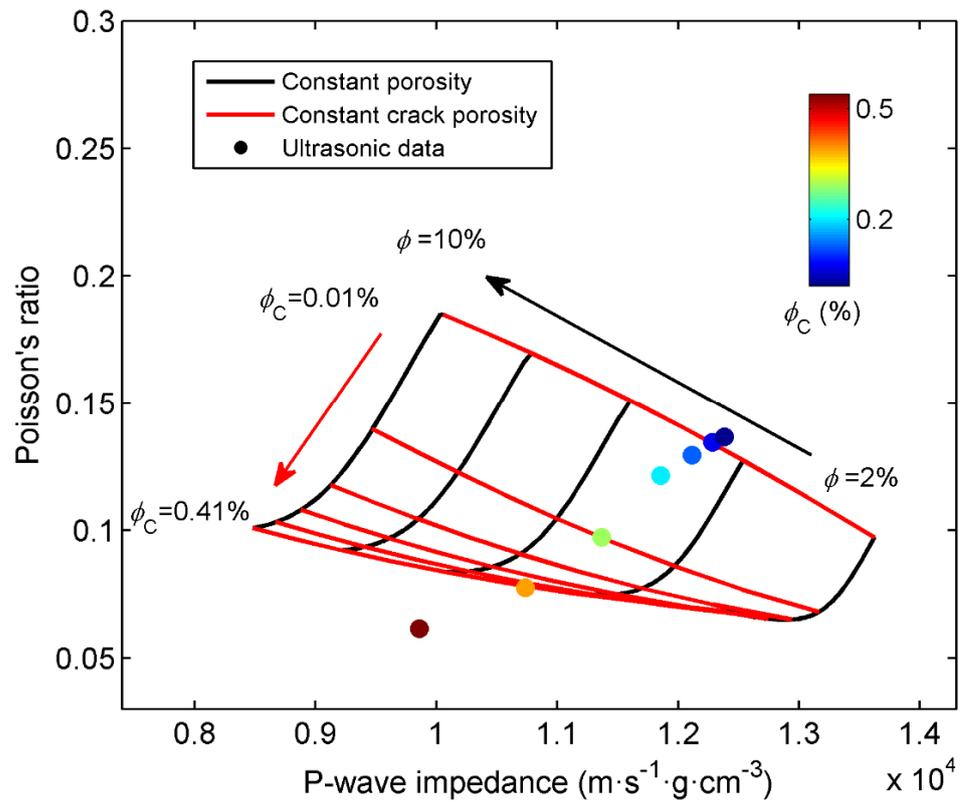
Figure 13. Ultrasonic data and corresponding RPT. The color bar indicates the microcrack porosity.
