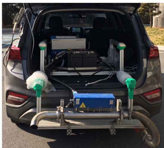
Figure 1. Example of the PEMS equipment installed on the test vehicle.
