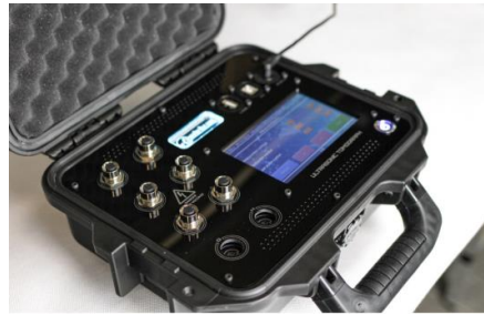
Figure 3. The developed 64-channel reflective ultrasound tomography.
