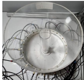
Figure 4. The experimental setup. The circular tank with 16 transducers and a cylinder phantom placed in its centre is filled with water during experimentation.
