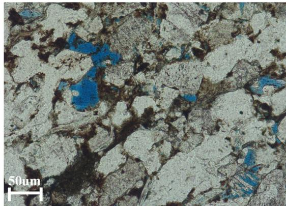
Figure 5. Thin section image of a tight sandstone.
