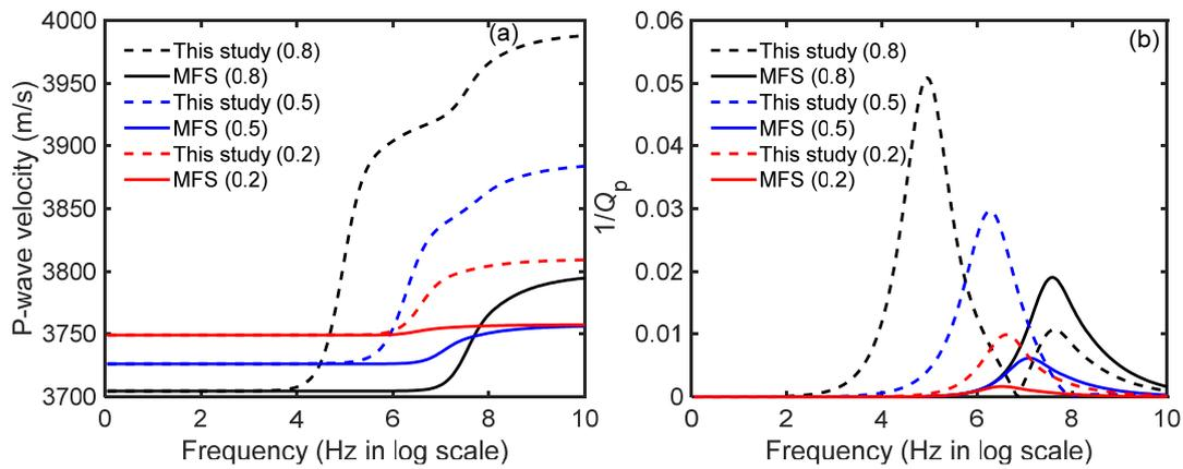
**Figure 2.** P-wave velocity (a) and attenuation (b) of the present and MFS models. The number between parentheses indicates water saturation.
