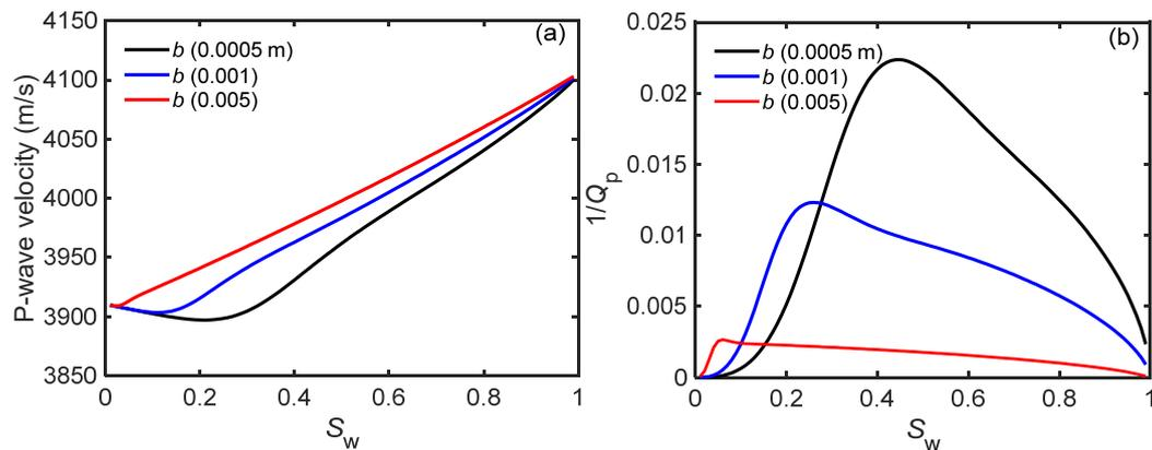
**Figure 4.** P-wave velocity (a) and attenuation (b) of the present model as a function of water saturation for different values of the outer diameter.
