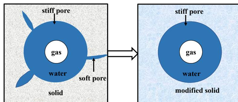
**Figure 1.** A new model based on a reformulated modified frame squirt flow (MFS) model with the White theory. The effects of squirt flow occurring between soft and stiff pores in the water-saturated host medium are incorporated by using an equivalent host medium of a modified solid (the MFS model). On the other hand, the White theory describes the anelasticity due to the patchy saturation of the immiscible fluid mixture.
