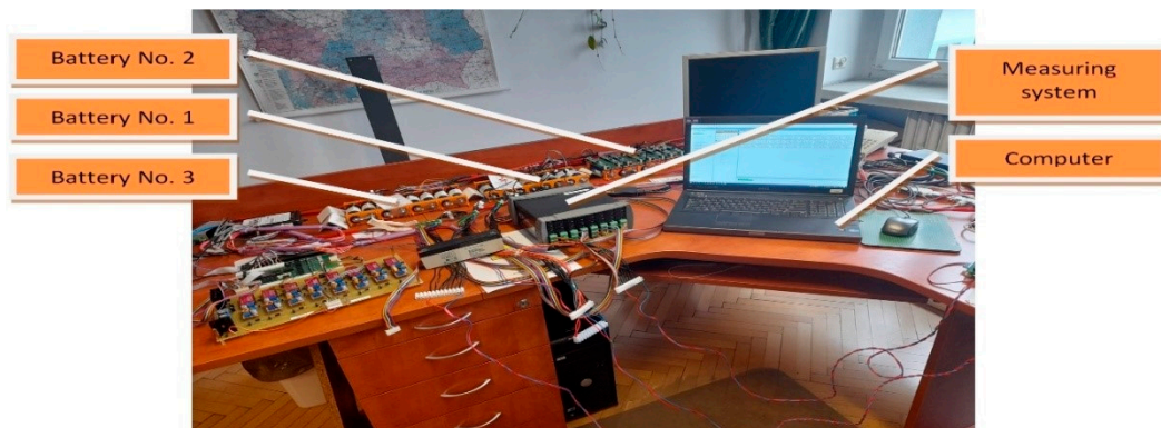
Figure 12. General view of test stand under room conditions (No. 1—with battery to cell active BMS, No. 2—with cell to battery active BMS, No. 3—with passive BMS).
