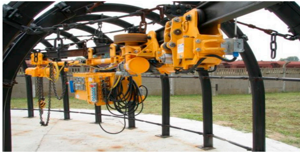
Figure 3. Operation of a suspended battery vehicle (PCA-1).
