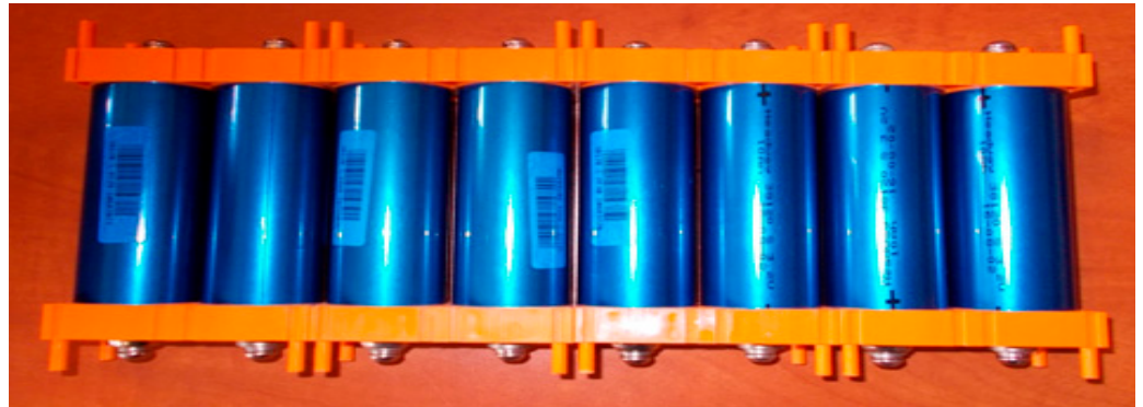
Figure 5. Battery pack arranged of eight lithium-iron-phosphorous (LiFePO 4 ) cells for testing.
