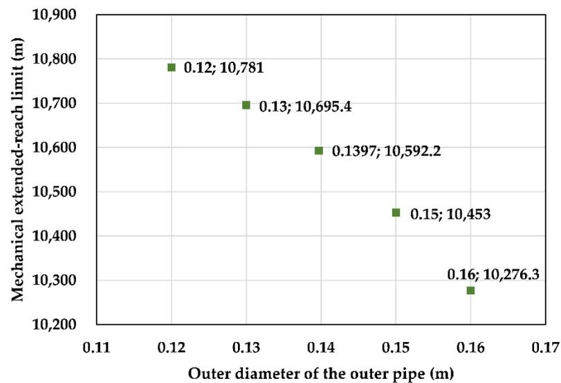
Figure 9. Effect of the outer diameter of the outer pipe on the mechanical extended-reach limit.
