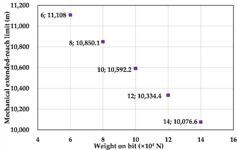
Figure 11. Effect of the weight on bit on the mechanical extended-reach limit.
