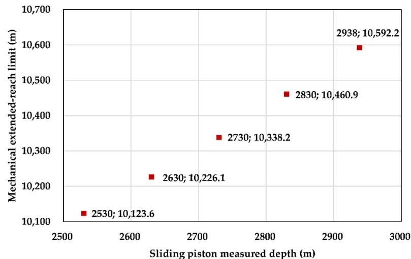
**Figure 8.** Effect of the sliding piston measured depth on the mechanical extended-reach limit.
