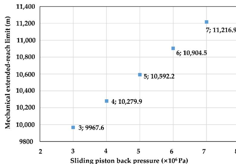
**Figure 7.** Effect of the sliding piston back pressure on the mechanical extended-reach limit.
