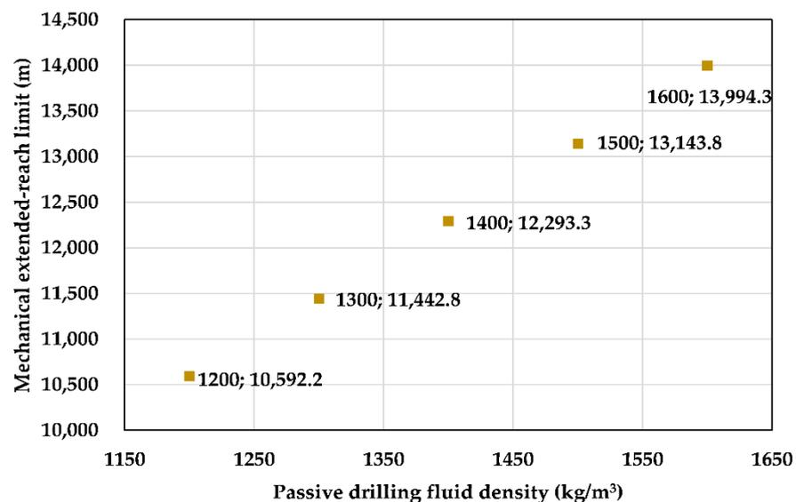
Figure 10. Effect of the passive drilling fluid density on the mechanical extended-reach limit.
