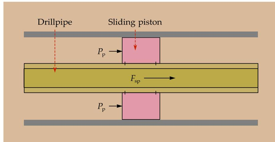
Figure 4. Schematic of a pump-in downhole tool.
