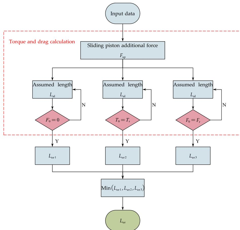
**Figure 5.** Calculation procedure of the mechanical extended-reach limit of the dual-channel drillpipe drilling.
