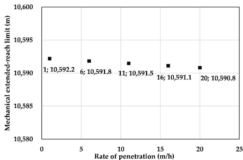
Figure 12. Effect of the rate of penetration on the mechanical extended-reach limit.
