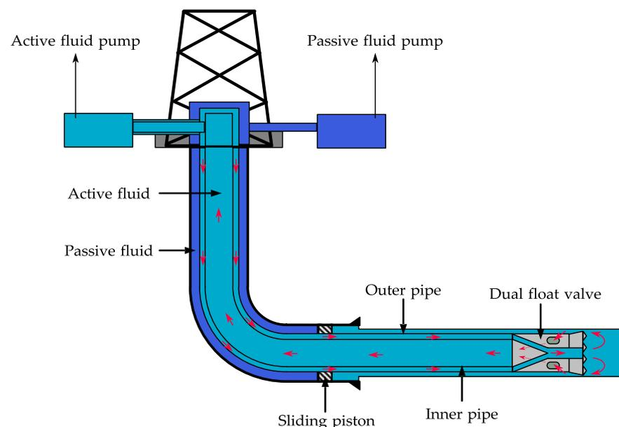
**Figure 1.** Schematic overview of dual-channel drillpipe drilling system.
