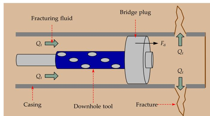
Figure 3. Schematic of a pump-in downhole tool.
