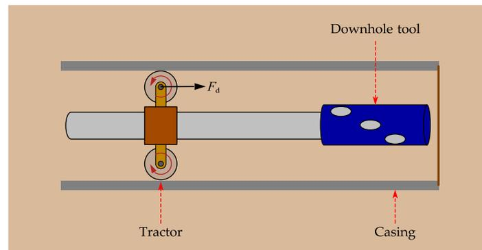
Figure 2. Schematic of a tractor.
