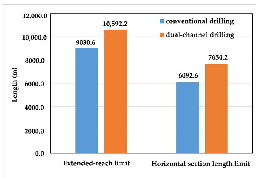
**Figure 6.** Comparison of conventional drilling to dual-channel drillpipe drilling.
