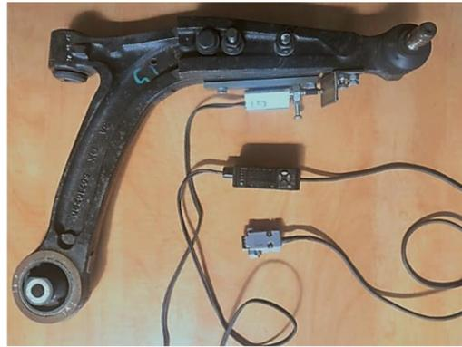
**Figure 6.** View of the measuring arm.
