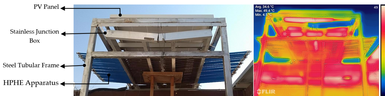
Figure 1. PV-HPHE apparatus isometric model (left) and captured infrared image (right) that were taken from the bottom surface in the Ecohouse, UTAS (formerly HCT), Muscat, Oman.
