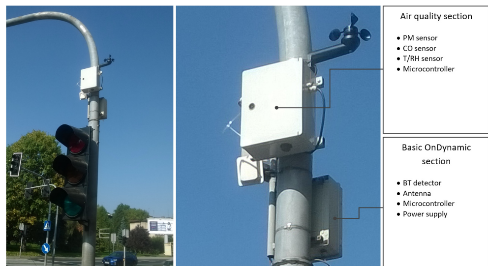
Figure 2. The view of the OnDynamic’s extended base station (T/RH—temperature and relative humidity; BT—Bluetooth).
