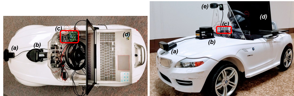
Figure 1. Ridon-Vehicle. Left: The top view of the Ridon Vehicle. Right: The profile view. (a) is a camera and (b) is a LIDAR for data acquisition. (c) is the motor control module. (d) is a laptop computer. (e) is a camera to take first-person-view videos for the platform.
