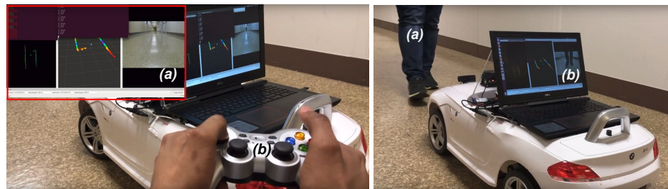
Figure 21. Rviz screen with multiple ROS nodes to use sensor packages. (Left): Remote control. (a) A screenshot of the ROS Visualization and our remote control ROS node. (b) A remote controller in action. Video: https://youtu.be/Vuj5jBDjNVs (accessed on 18 November 2021) . (Right): (a) An object. (b) ROS topic viewers from the LIDAR and the front camera. Video: https://youtu.be/vomTh7FF7K8 . (accessed on 18 November 2021)
