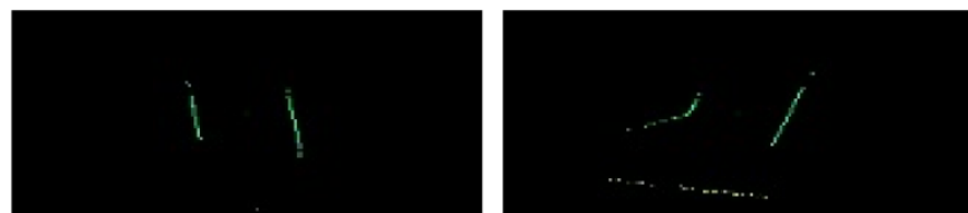
Figure 19. Examples of images collected from the LiDAR. Point clouds are projected into a bird-eye view 2D plane.
