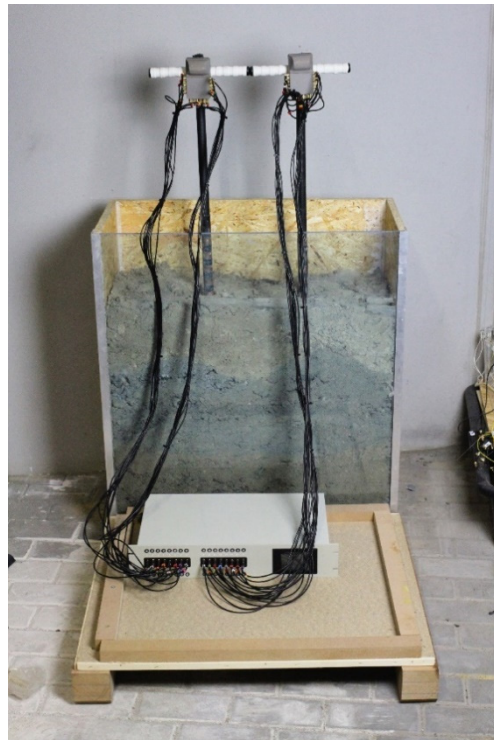
Figure 5. Laboratory model with two multi-sensor electrodes during electrical tomography measurements.
