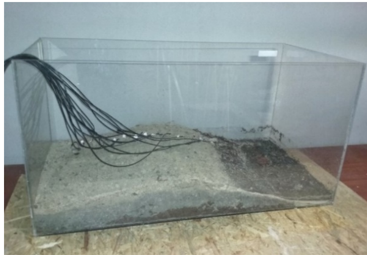
Figure 16. A laboratory model of the flooded embankment with 16 measuring sensors.
