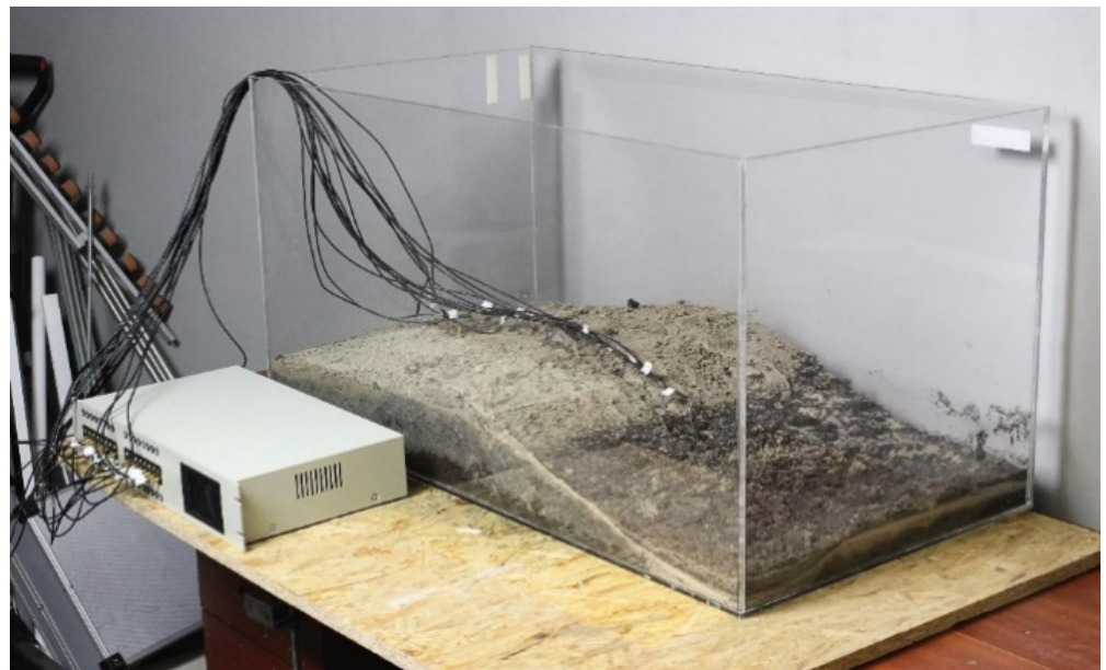
Figure 4. Laboratory system with measuring electrodes during measurements with an electrical tomograph.
