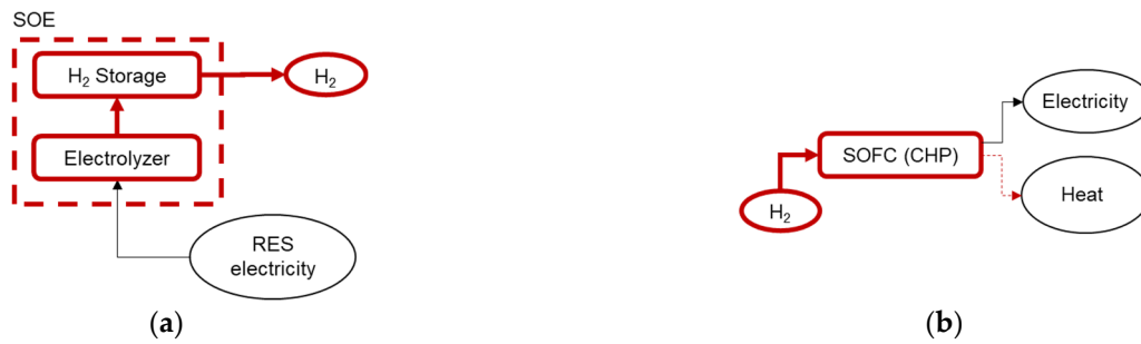
Figure 2. r-SOC working diagram used for the optimization model: (a) SOE mode; (b) SOFC mode.
