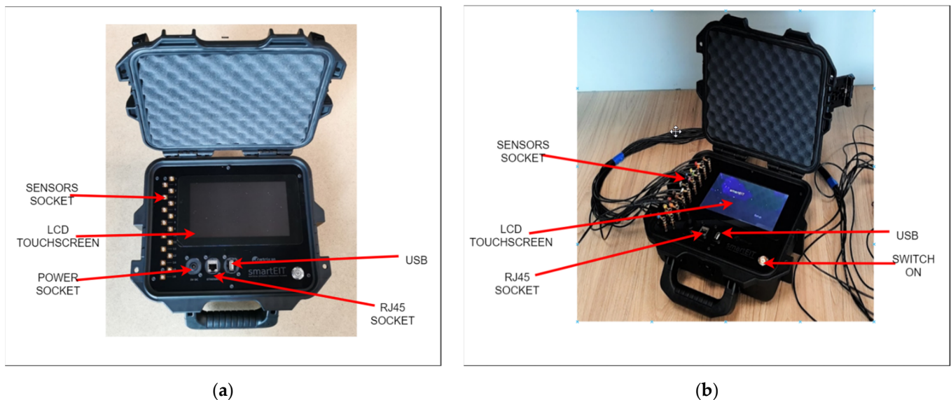
Figure 2. Photos showing the view of the SmartEIT scanner placed in the housing on the left (a) and the device connected to the probes and working—on the right (b).
