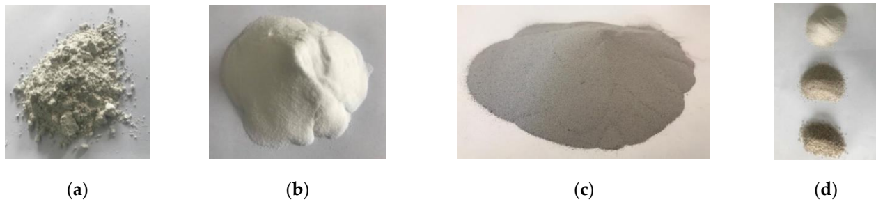
Figure 1. Raw materials used for the design of AAMs with M3DPWP: (a) GGBFS; (b) WG; (c) M3DPWP; (d) aggregates.
