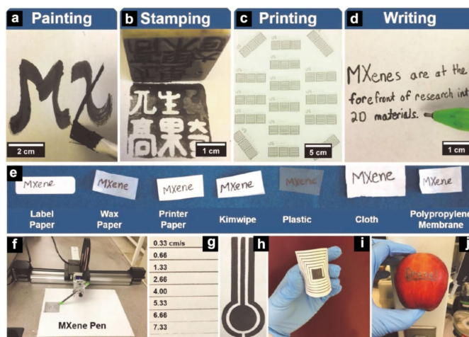
Figure 8. (a–e) Written MXene on various substrates via various ways, (f,g) using the automatic drawing tool of AxiDraw for patterning by using the \text{Ti}_3\text{C}_2 inks, (h,i) versatile patterning using AxiDraw, and (j) a demonstration of MXene inks drawn on an apple [81].
