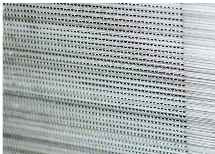
**Figure 1.** Inside configuration of printed circuit heat exchanger (PCHE) [13].
