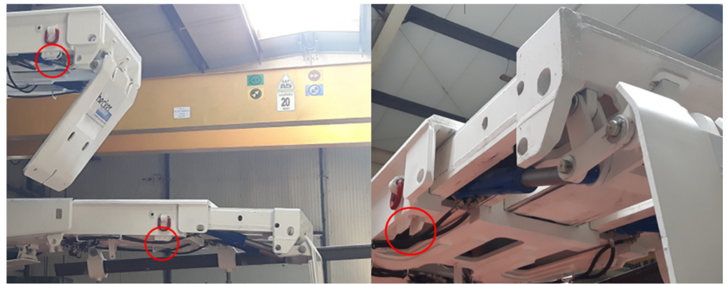
Figure 3. The BW 24/44 POz shield support with marked space for the SSMS-S sensor.
