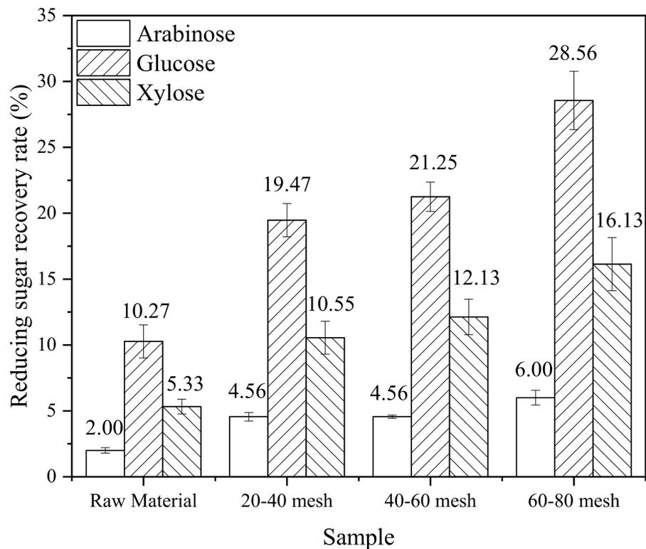
Figure 4. Enzymatic hydrolysis recovery rates of monosaccharides after thread rolling and sieving.
