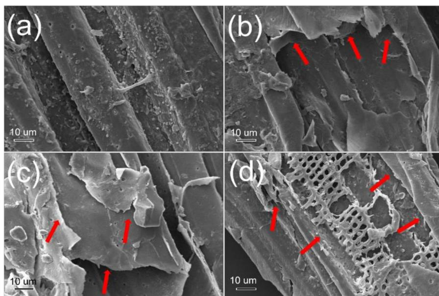
**Figure 2.** SEM images of the raw material and thread rolling treated fibers ((a) Raw materials; (b) 20–40 mesh enzymatic residue; (c) 40–60 mesh enzymatic residue; (d) 60–80 mesh enzymatic residue).
