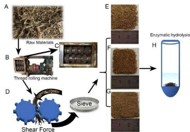
**Figure 1.** Mechanism of the thread rolling pretreatment ((A) Corn stalks and sugar cane bagasse raw material; (B,C) Thread rolling machine; (D) Schematic diagram of the mechanism of thread rolling; (E) 20–40 mesh sample; (F) 40–60 mesh sample; (G) 60–80 mesh sample; (H) Enzymatic hydrolysis reactor).
