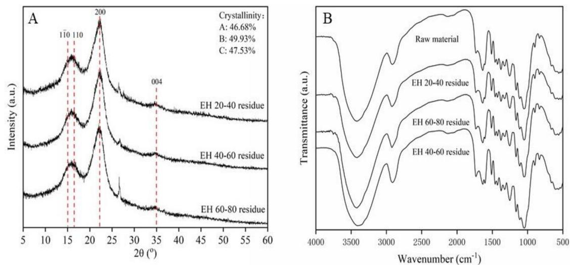
**Figure 5.** (A) XRD patterns and (B) FT-IR spectra of mixed corn stalks and sugar cane bagasse samples treated by thread rolling and enzymatic hydrolysis residues (EH means enzymatic hydrolysis).
