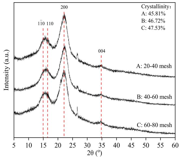
Figure 3. XRD patterns of the thread rolled samples with various meshes.
