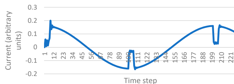
Figure 6. Circuit current for an example of the implementation of the simple partial discharge circuit.
