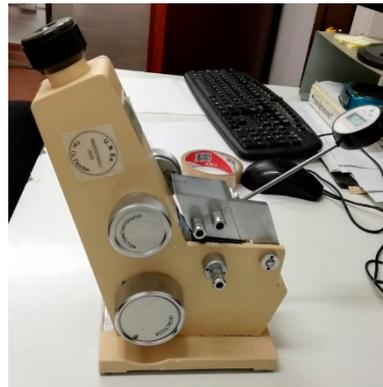
**Figure 5.** Krüss AR4 refractometer used in the experiments.
