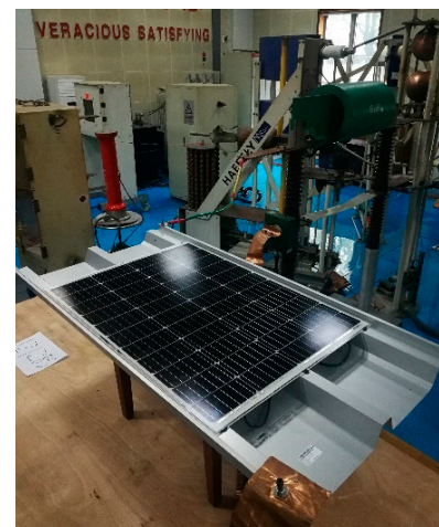
Figure 11. Lightning current withstand performance experiment (a) Schematic diagram of experimental platform; (b) Layout of experimental setup.
