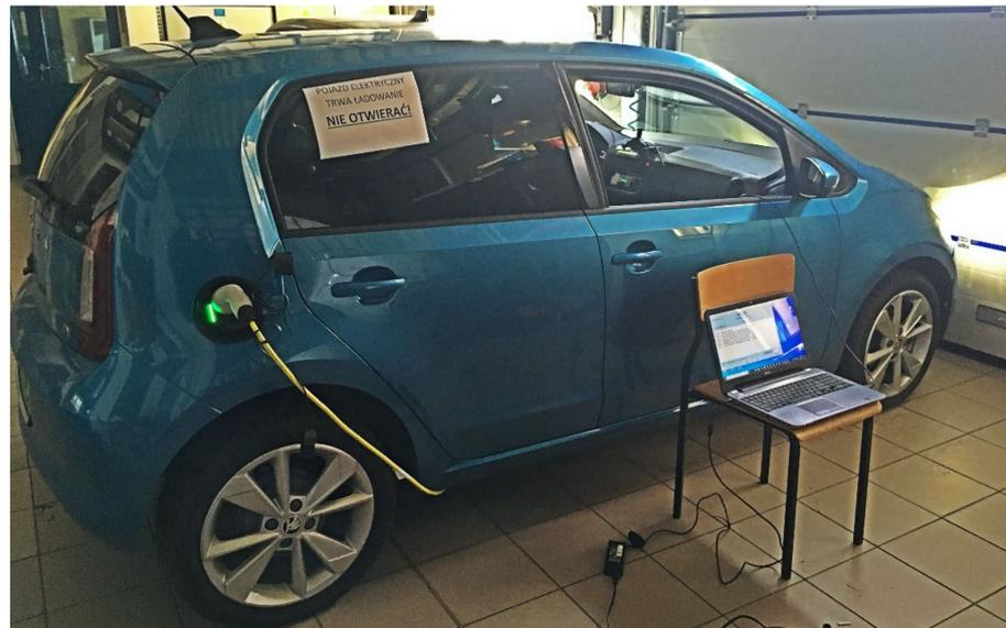
Figure 3. Vehicle charging setup.
