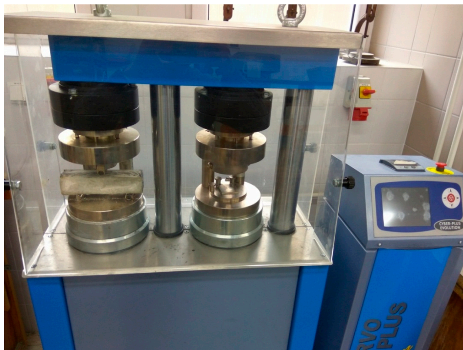
Figure 11. Hydraulic press Servo-Plus Evolution E183.
