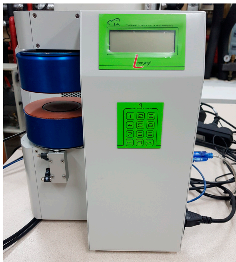
Figure 14. FOX 50: thermal conductivity measurement apparatus.
