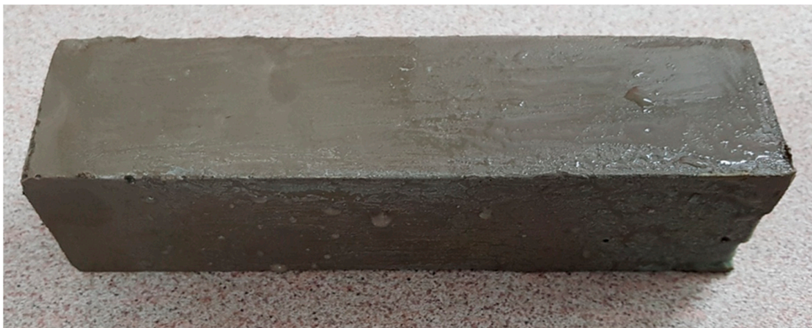
Figure 10. An example of a standard beam subjected to strength testing.
