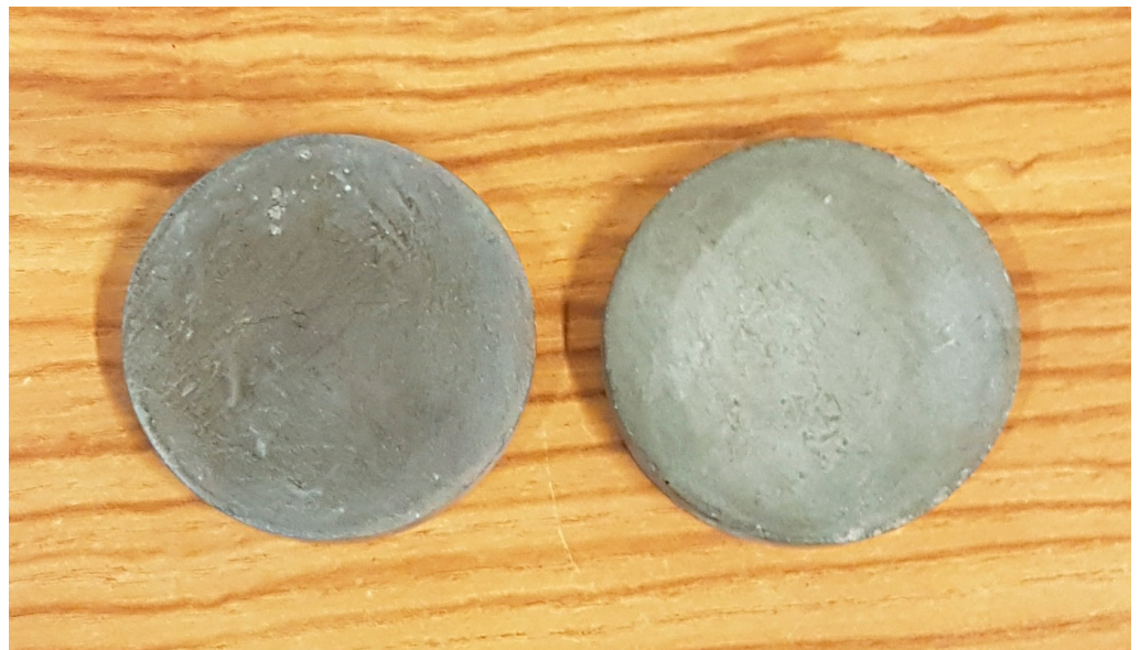
Figure 13. An example of a prepared round samples subjected to thermal conductivity testing.
