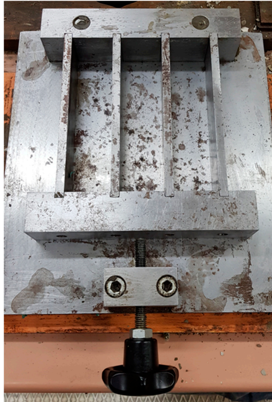
Figure 9. The molds for the beams.
